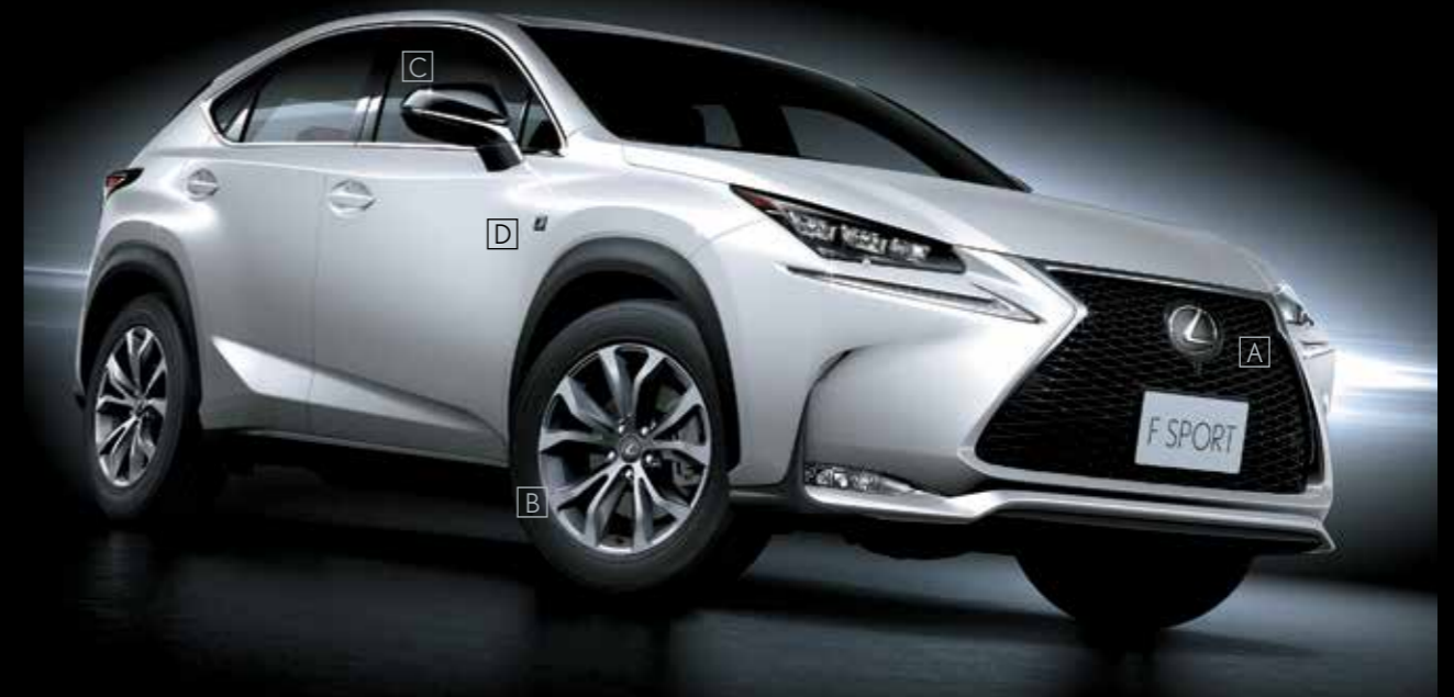
A/ Front Mesh Grille & Front Bumper Distinctive honeycomb spindle grille and unique bumper for a bold and assertive design statement.
